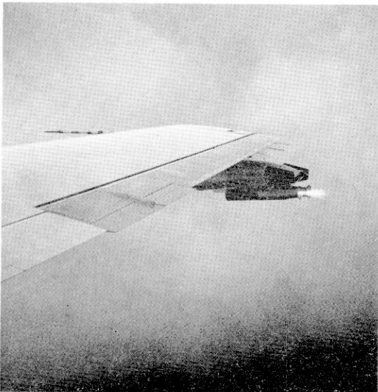
Fig. 3. Steady-state flame type generator in operation during the Lake-Effect Snow Project. Photo by B. Patten.
