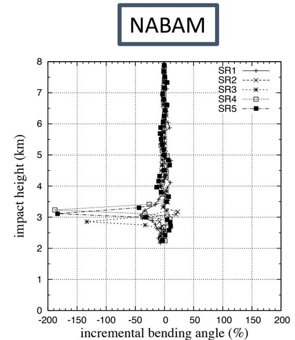
Differences between the observed and simulated bending angle profiles (in percentage) for five profiles likely affected by atmospheric super-refraction conditions with the use of NBAM and NABAM forward operators.
