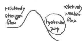
As relatively stronger flow goes over mountain, a strong adjustment is needed  $\Rightarrow$  a shock wave, or hydraulic jump occurs.
