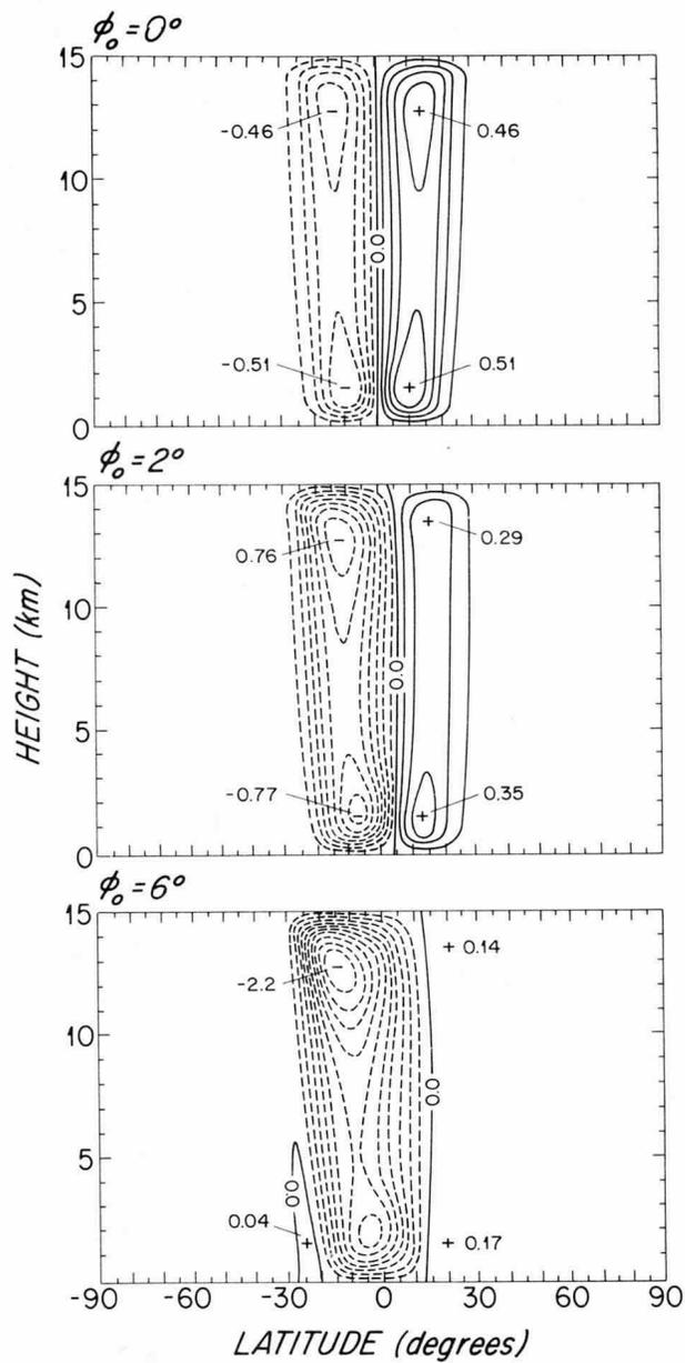
FIG. 9. Numerical model results for  $\psi$  for (a)  $\phi_0 = 0^\circ$ , (b)  $\phi_0 = 2^\circ$ , and (c)  $\phi_0 = 6^\circ$ . Units are in  $10^{10} \text{ kg s}^{-1}$  and the contour interval is  $0.1 \times 10^{10} \text{ kg s}^{-1}$  for (a) and (b); twice this value for (c).
