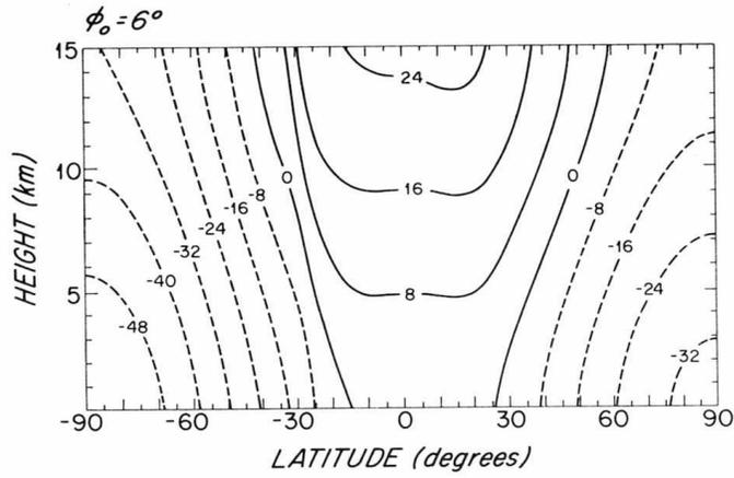
FIG. 12. The calculated temperature field for  $\phi_0 = 6^\circ$ . The values correspond to departures from  $\theta = 300$  K. The contour interval is 8 K.
