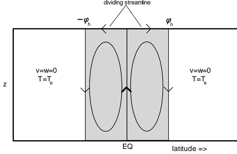
Figure 3: Schematic. AMC region is shaded, TE unshaded. (Note that the edges of the Hadley cell do not need to be vertical.)
