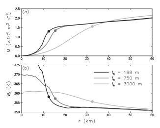
FIG. 4. Properties at the top of the boundary layer (z = 1.1 km) from simulations that use different values for  $l_h$ , as indicated by the legend (using  $l_v = 200$  m): (a) angular momentum (M), and (b) equivalent potential temperature ( $\theta_e$ ). Dots indicate the location of  $v_{\rm max}$  in these simulations.
