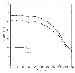
FIG. 3. Maximum azimuthal velocity ( $v_{\text{max}}$ , solid) and maximum gradient wind ( $v_{g,\text{max}}$ , dashed) from simulations that use different values for  $l_h$  (using  $l_v = 200 \text{ m}$ ).
