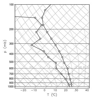
FIG. 1. The thermodynamic sounding used for this study. Dots are the data used in the simulations by RE87, and lines illustrate interpolation (between points) and extrapolation (downward from the lowest model level) to initialize higher-resolution simulations.
