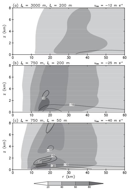
FIG. 5. Output from simulations that use different specification of the turbulence length scales: (a)  $l_h = 3000$  m and  $l_v = 200$  m; (b)  $l_h = 750$  m and  $l_v = 200$  m; (c)  $l_h = 750$  m and  $l_v = 50$  m. Azimuthal velocity is shaded and radial velocity is contoured every  $10 \text{ m s}^{-1}$  with negative contours dashed and the zero contour excluded. The minimum value of u is listed at the top of (a)–(c).
