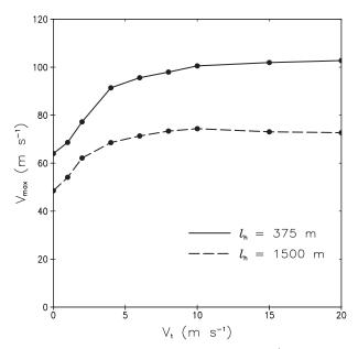
FIG. 7. Maximum azimuthal velocity ( $v_{\text{max}}$ , m s<sup>-1</sup>) from simulations that use different values for terminal fall velocity ( $V_t$ , m s<sup>-1</sup>) using  $l_h = 375$  m (solid) and  $l_h = 1500$  m (dashed).
