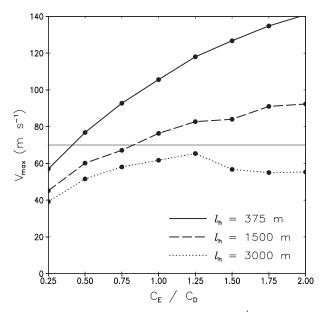
FIG. 6. Maximum azimuthal velocity ( $v_{\rm max}$ , m s<sup>-1</sup>) from simulations that use different ratios of surface exchange coefficients for entropy and momentum,  $C_E/C_D$ , using  $l_h=375$  m (solid),  $l_h=1500$  m (dashed), and  $l_h=3000$  m (dotted). The gray line denotes 70 m s<sup>-1</sup>, which is the approximate maximum intensity observed for this sea surface temperature.
