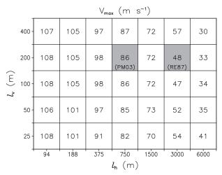
FIG. 2. Maximum azimuthal velocity ( $v_{\text{max}}$ , m s<sup>-1</sup>) from simulations that use different values for  $l_h$  and  $l_v$ . Shaded boxes denote settings used by RE87 and PM03.
