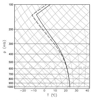
FIG. 9. Thermodynamic soundings used for sensitivity analysis: a reversible sounding (solid) and a pseudoadiabatic sounding (dashed). Both soundings are saturated, and both have the same equivalent potential temperature at the surface as the control sounding.
