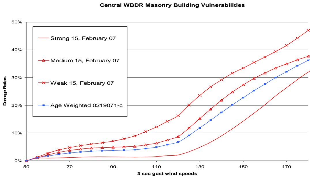
**Figure 3. Weighted masonry structure vulnerabilities in the Central wind bone debris zone**
