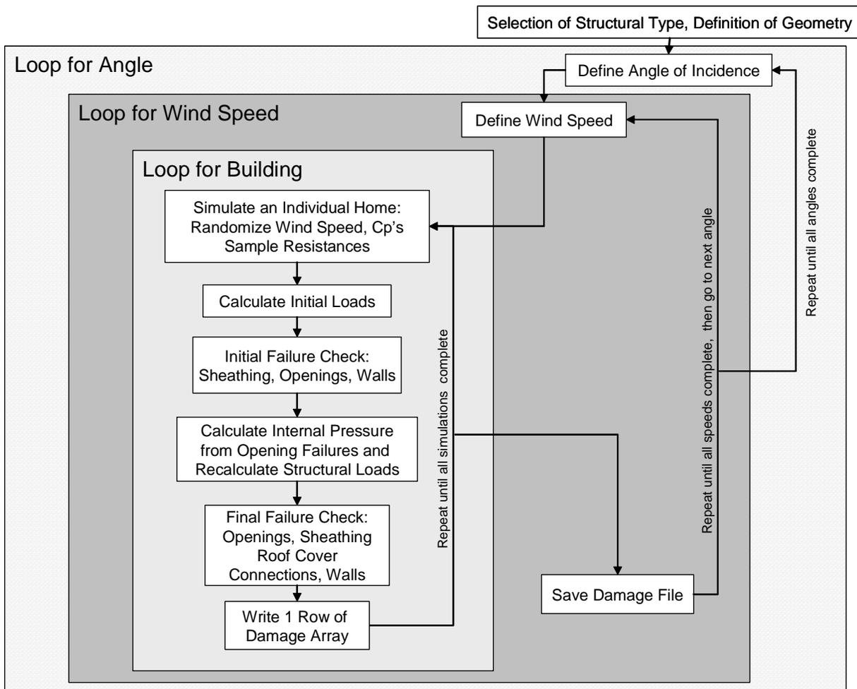
**Figure 28. Monte Carlo Simulation Procedure to Predict Damages**
