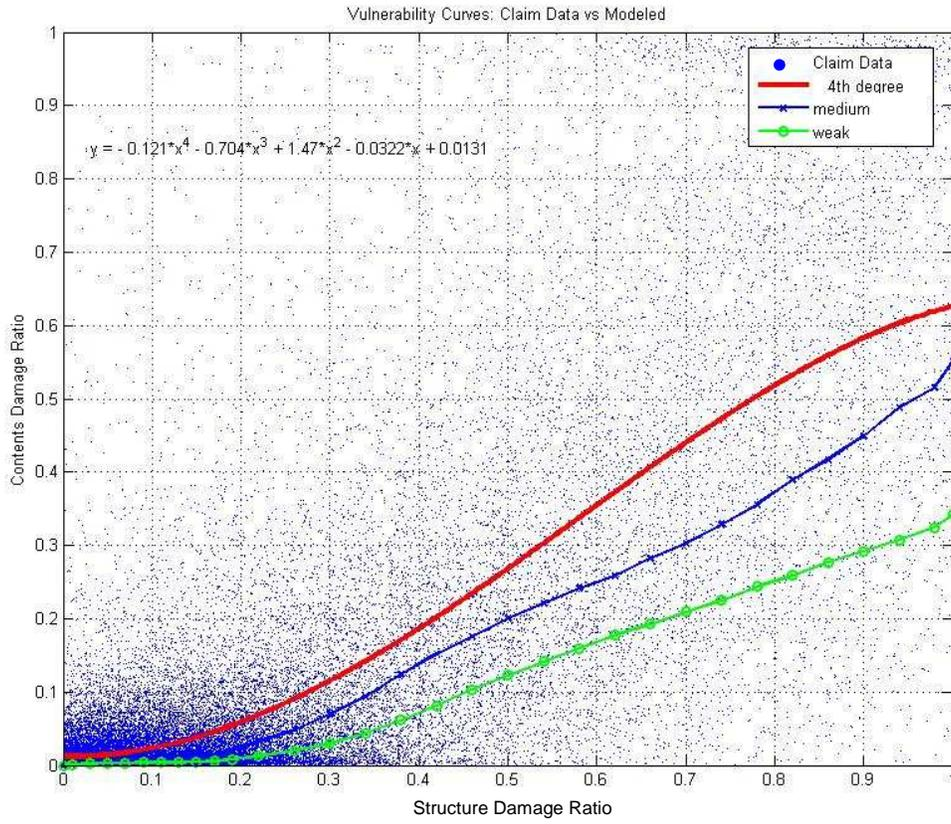
**Figure 39. Modeled vs. Actual Relationship between Structure and Content Damage Ratios**
