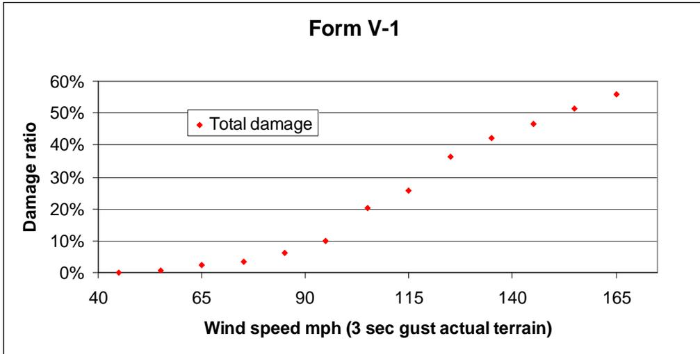
**Figure 31. Total damage vs. wind speed**
