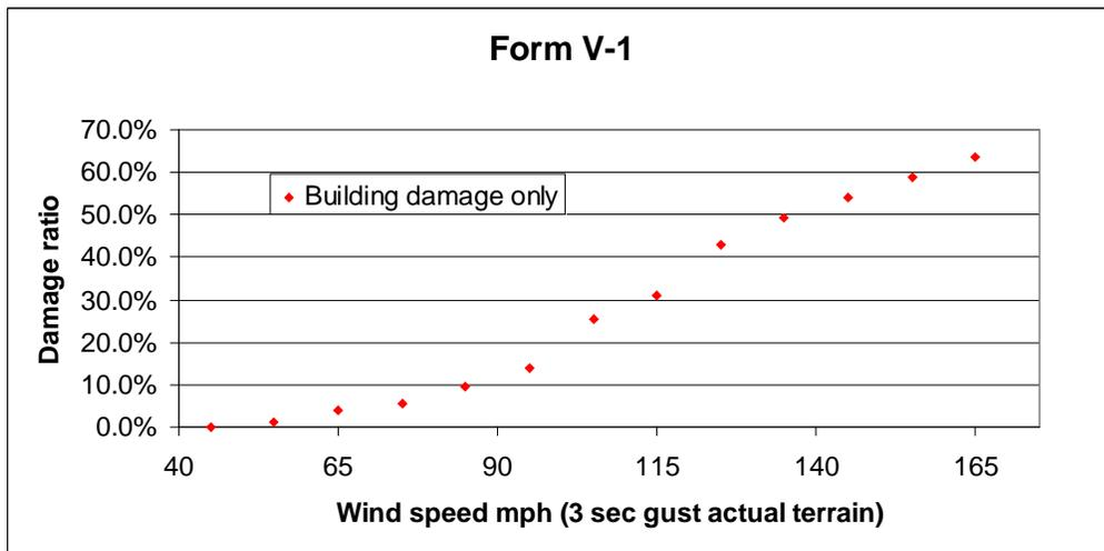
**Figure 32. Building damage vs. wind speed**
