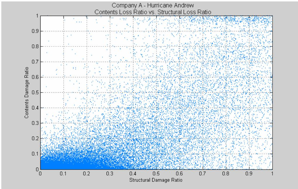
**Figure 30. Company A, Hurricane Andrew structure vs. contents losses**
