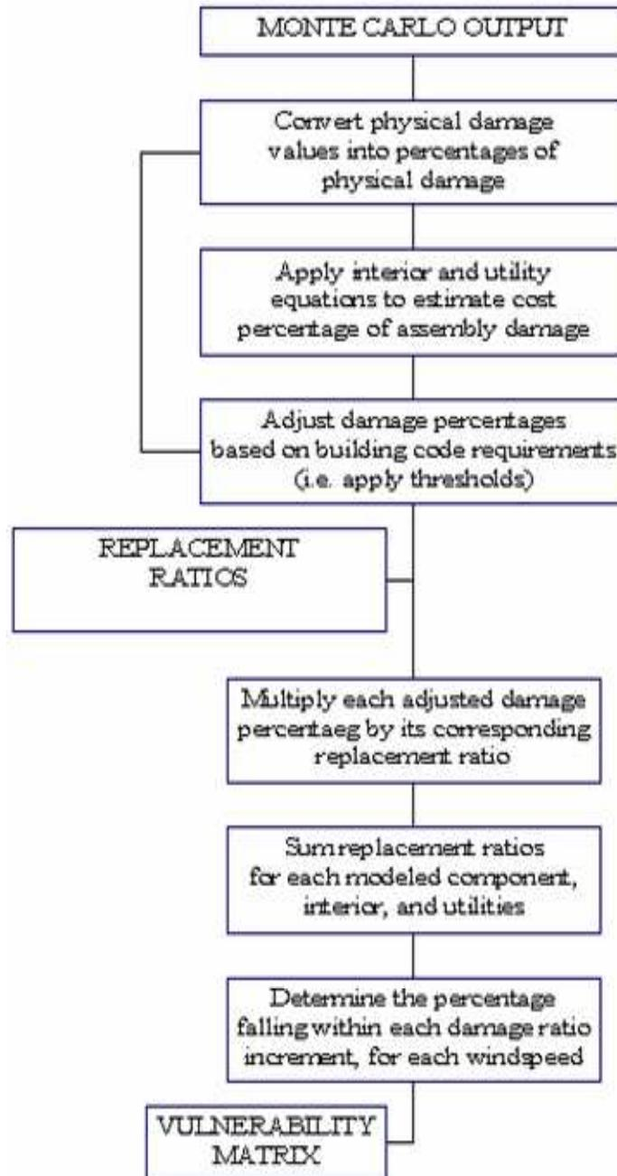
Figure 29. Procedure to create vulnerability matrix
