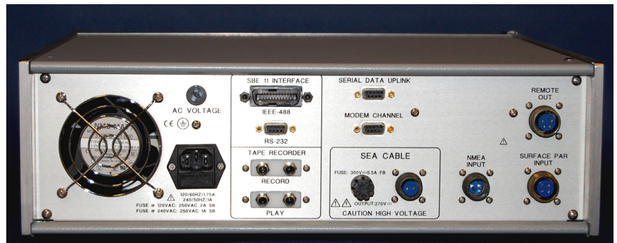
Back Panel – connectors and fuses
