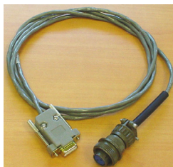
NMEA Input Interface test cable
