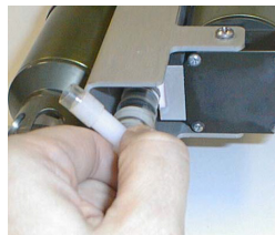
Rotate C Duct clockwise
