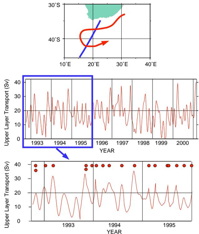
Fig. 2: (top) Schematic of the Agulhas Current retroflexion. (center) Baroclinic transport from the surface to the 10°C isotherm across a selected TOPEX/Poseidon altimeter ground track from the coast to 40°S. (blue line in top panel). (bottom) Baroclinic transport between 1993 and 1995 showing a strong correspondence between ring shedding (red circles) and maximum transport values.
