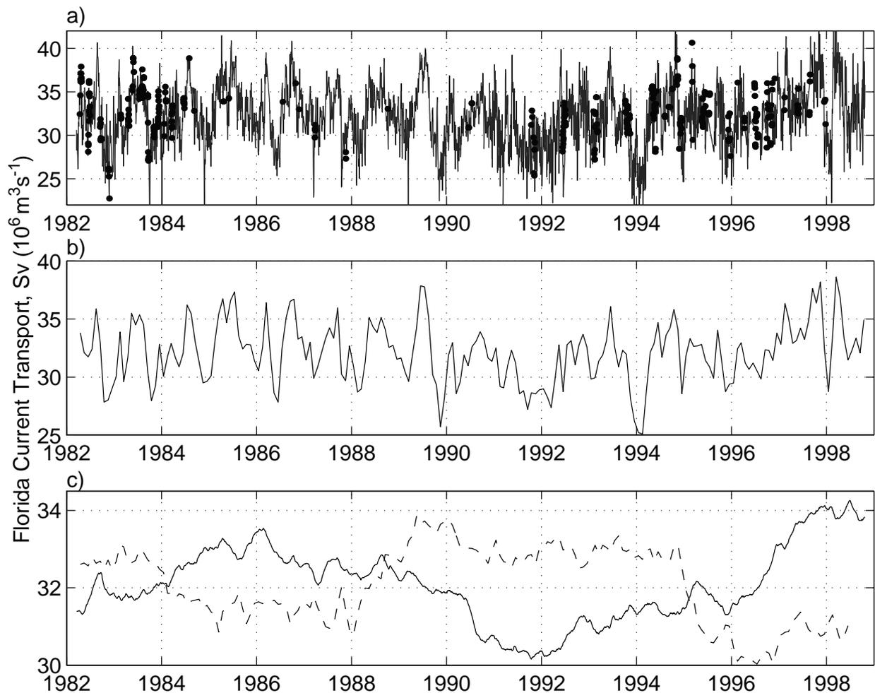
Fig. 4: Time series of Florida Current transport inferred from the cable voltages including (a) the daily transport values (blue line), (b) the monthly average transport, and (c) the two year running means of the daily transport values (solid line). Panel (c) also includes a monthly mean NAO index (Hurrell, 1995) (dashed line). Panel (a) includes in situ observations of Florida Current transport obtained on small boat cruises (solid circles).
