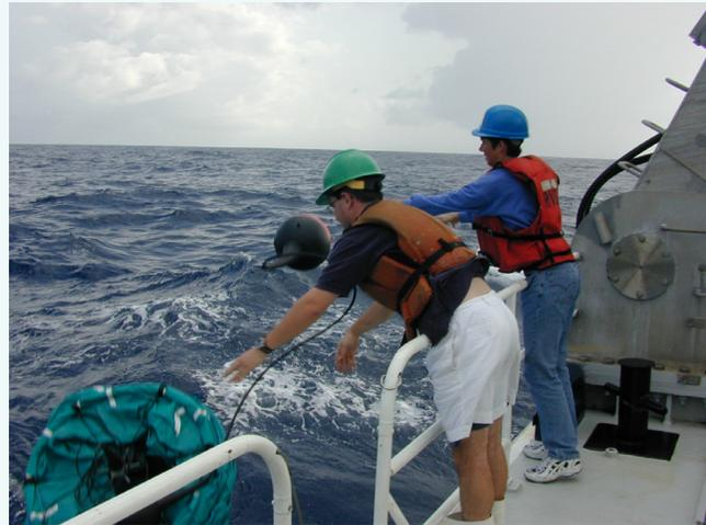
*Deployment of a drifting buoy.*
