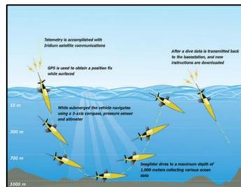
An underwater glider is an autonomous underwater vehicle (AUV) that uses small changes in buoyancy together with wings to propel itself by converting vertical motion into horizontal motion. Thanks to a very small consumption of energy, underwater gliders have longer ranges when compared to other AUVs, being able to measure several ocean parameters during months, including temperature, salinity, and dissolved oxygen.
