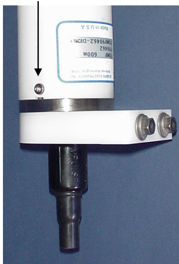
Detail - Battery/connector end cap
