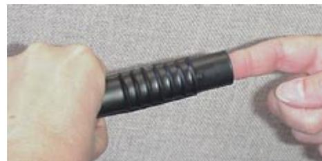
4. *Standard XSG/AG connectors only:* Align the *bump* on the cable boot or dummy plug with the large pin on the bulkhead connector, and align the sockets with the pins.
