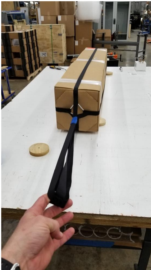
Figure 5. ALTO float with over-the-side launch harness in hand.
