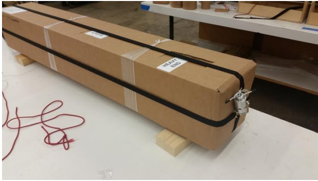
Figure 4. ALAMO ready for sea launch showing soluble strap link at base.
