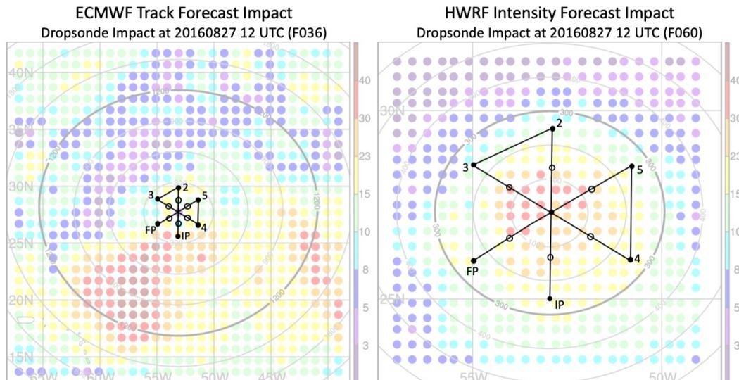
*Figure 1. P-3 Synoptic Flow pattern for a TC mission flown on 27 Aug 1200 UTC designed to impact the forecast for 29 Aug 0000 UTC. The plots show hypothetical reductions in (left) ECMWF position variance and (right) HWR intensity variance due to assimilating GPS dropsonde data at each horizontal location. Warmer colors denote areas where GPS dropsonde data could most effectively reduce variance amongst the ensemble members.*
