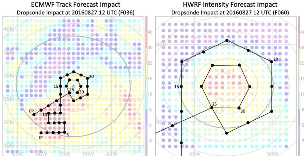
Figure 2. G-IV Synoptic Flow pattern for a mission flown in a TC on 27 Aug 1200 UTC designed to impact the forecast for 29 Aug 0000 UTC. The plots show hypothetical reductions in (left) ECMWF position variance and (right) HWRf intensity variance due to assimilating GPS dropsonde data at each horizontal location. Warmer colors denote areas where GPS dropsonde data could most effectively reduce variance amongst the ensemble members.
