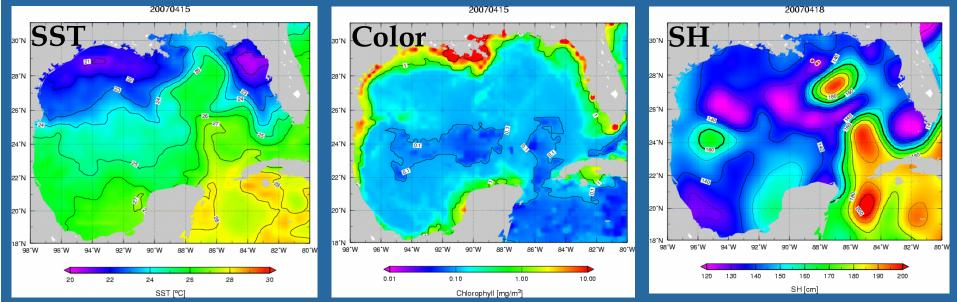
**Sea surface temperature:** Microwave, objective analyzed daily data, 25km spatial grid from TMI and Aqua. These data are not affected by cloud coverage. *Source: Remote Sensing Systems*.
