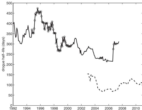
FIG. 6. Drogue half-life as a function of deployment date, calculated in a 1-yr sliding window for the original-design drifters (solid) and for the redesigned minidrifter (dashed); values are not shown if there were fewer than 50 drifters of that type deployed in the 1-yr window. Open circles indicate values for which more than half the drifters died with the drogues still attached.
