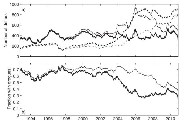
FIG. 4. (a) Number of drifters with (solid) and without (dashed) drogues, *before* (thin) and *after* (thick) automatic drogue reanalysis. (b) Fraction of drifters with drogues *before* (thin) and *after* (thick) reanalysis.
