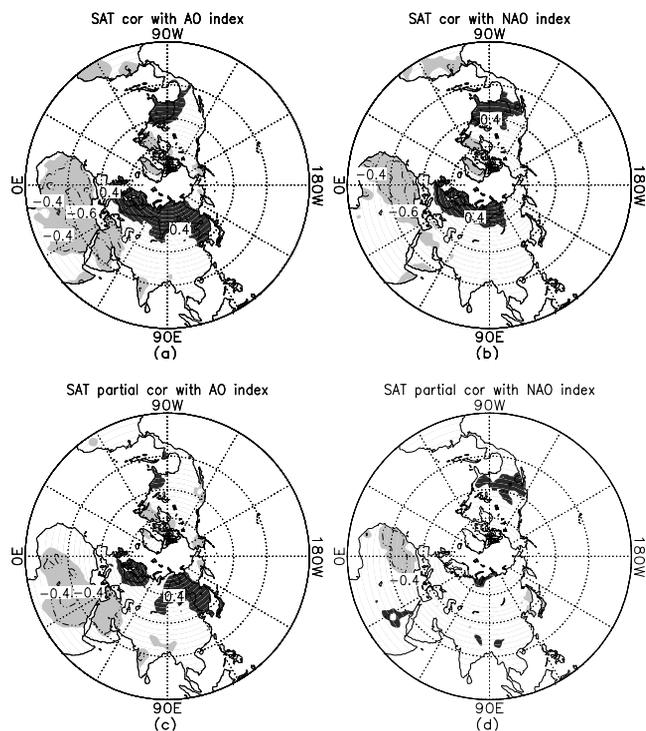
**Figure 2.** Correlations of surface air temperature over land with detrended (a) the AO index, and (b) the NAO index; The contour interval is  $-0.6, -0.4, 0.4, 0.6$ ; The shaded areas denote correlations exceed 95% confidence level t-test; (c), (d), the same as (a), (b) but for the partial correlations.
