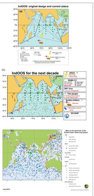
FIGURE 2 | (a) IndOOS original design and current status. The original IndOOS design comprises the RAMA, Argo, XBT network, surface drifting buoys, and tide gauge components. (b) The proposed evolution of IndOOS (from the IndOOS decadal review led by IORP, to be published in 2019).
