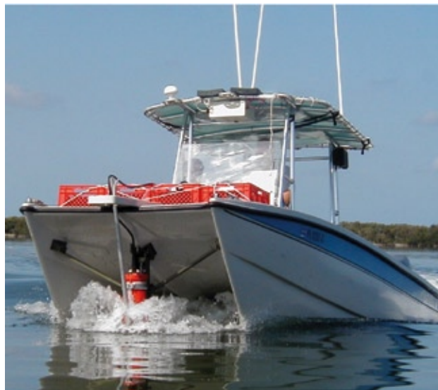
Fig. 2- The R/V Virginia Key measuring volume transports through a channel connecting Fla Bay inner basins. The Virginia Key was configured specifically for shallow water research.
