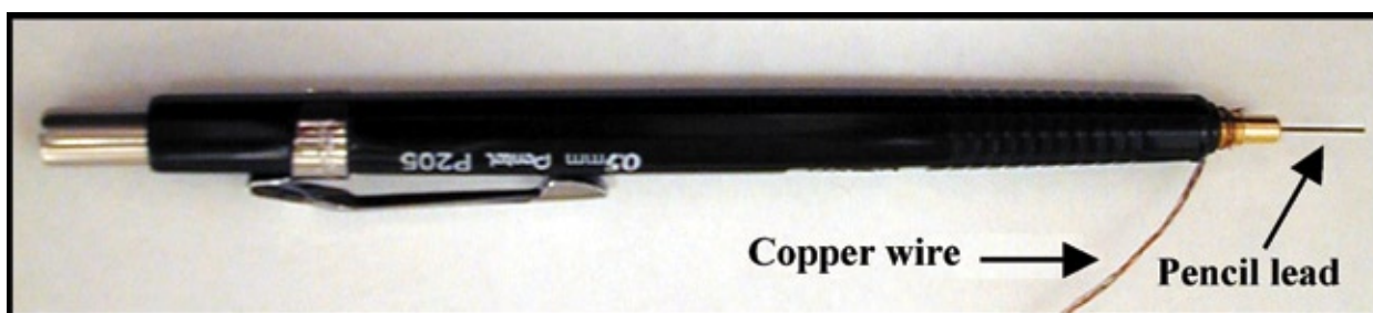
Fig. 1- DNA captured by molecular probes are detected by a carbon electrode (modified mechanical pencil).
