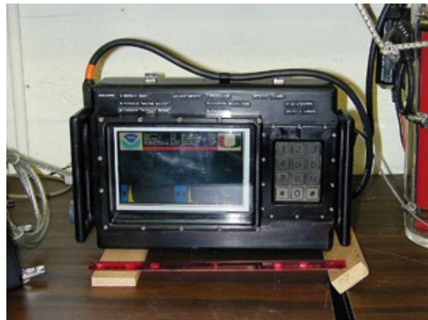
Fig. 1- The above picture shows the back of the camera system. The display shows information on internal temperature, exposure setting, gain, number of frames taken, and current operational status of the system. Images from each camera are shown in the display along with a real-time histogram of the images to help in setting system exposure. Just out of the screen on the right is the system battery. There is a connector on the right side of the case which allows another computer to be connected via Ethernet, to allow data transfer without opening the case.
