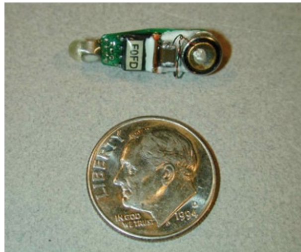
Fig. 1- Sample micro-acoustic tag (Battelle-PNNL Labs, Portland, OR) to be used in tracking the movements of juvenile snappers in the Western Sambo Ecological Reserve, Florida Keys National Marine Sanctuary.
