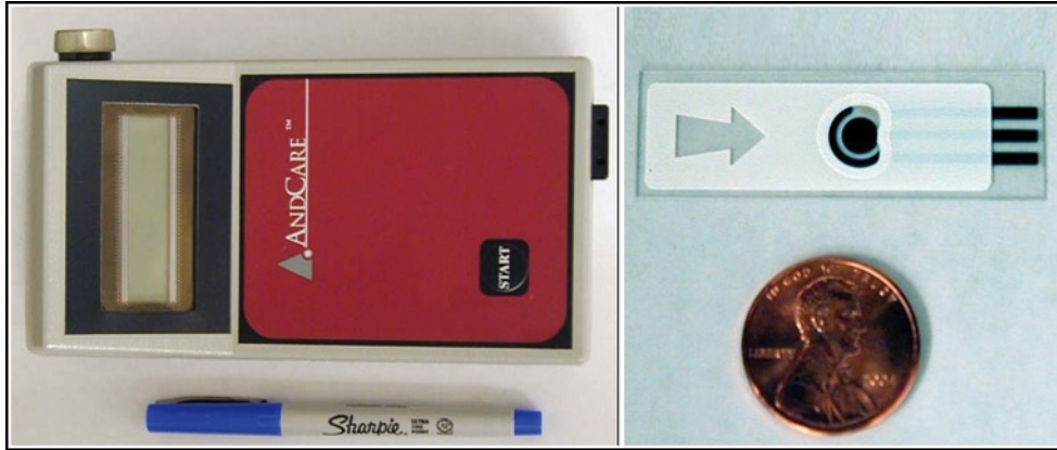
Fig. 2- Hand-held instrument and disposable sensors for detection of fecal bacteria and harmful algae ( www.alderon.com )
