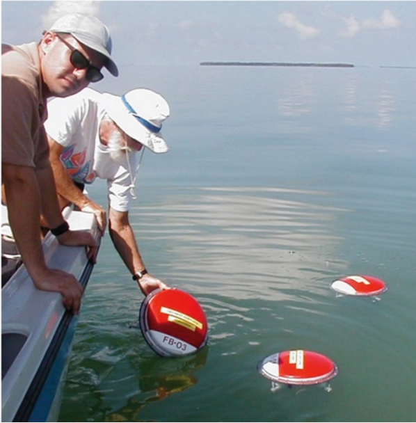
Fig. 1- These mini-drifters are designed for deployment in the very shallow waters of Florida Bay. They are tracked by both ARGOS satellite and GPS. This image shows the deployment of shallow water surface drifters designed for our study of inner basin circulation.
