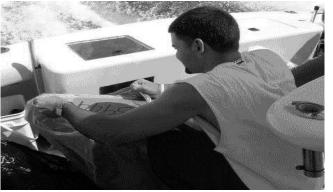
2. <u>DO NOT REMOVE</u> paper tape or cardboard. ONLY remove plastic wrap.
