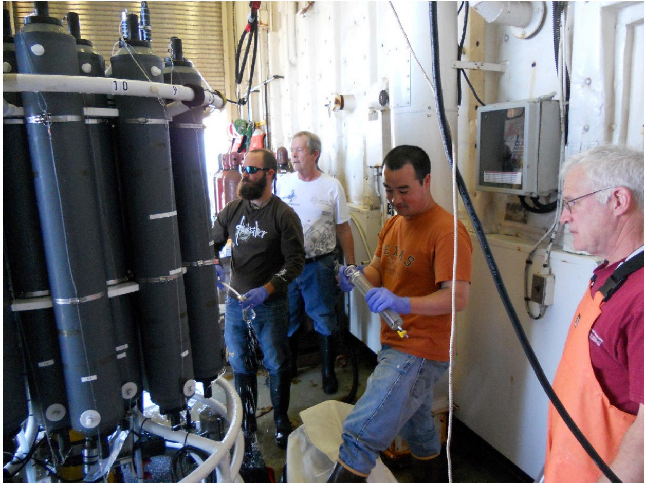
Figure 3: Sampling of the main sampling bottles is organized chaos with up to 8 persons subsampling the bottles with their own specialized containers. Since samples degrade or get contaminated at different rates after opening the bottles there is a designated order of sampling and rapid sampling is required. The skills of sampling are sometimes passed on over generations. Here, Eric Wisegarver (PMEL) is being trained to use large syringes to subsample for Freons while David Wisegarver (PMEL) is overseeing proper sampling procedures. In the background Andy Stefanick (AOML) is sampling for oxygen [the sunglasses are to avoid seeing unwanted bubbles in the sampling flasks...], while Bob Castle (AOML) is waiting for his sample for dissolved inorganic carbon. Gloves are worn to avoid contamination of samples for organic carbon in seawater taken later in the sampling sequence.
