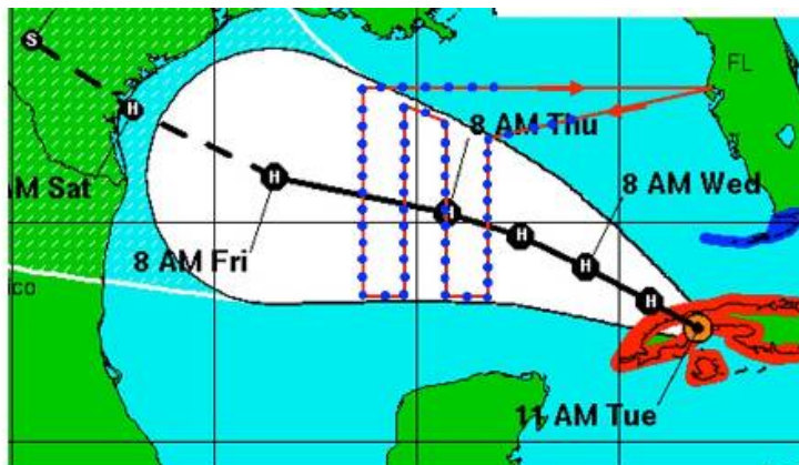
Figure OC-7: Track-dependent AXBT/AXCTD ocean survey. As for the Loop Current survey, a total of 60–80 probes would be deployed on a grid (blue dots).
