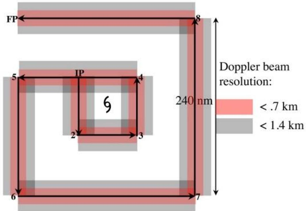
**Figure 1-2:** Doppler radar coverage for box-spiral pattern A. Pink region shows areas where vertical beam resolution is better than 0.7 km and gray regions delineate areas where vertical beam resolution is better than 1.4 km. Maximum extent of gray area is approximately 40 km from flight track, approximately the maximum usable extent of reliable airborne Doppler radar coverage. Flight distance in pattern above is 1280 nm, and flight time is 5.33 hours.
