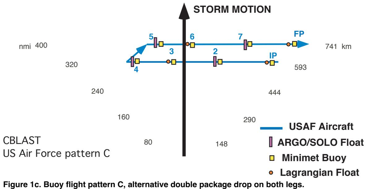
• Note 1. The US Air Force aircraft will also deploy GPS dropsondes at each buoy drop point along the track.
