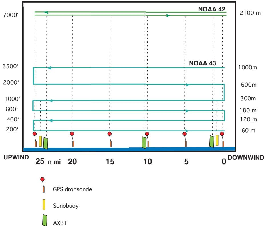
**Figure 6. CBLAST stepped descent pattern (racetracks) in upwind / downwind direction.**
