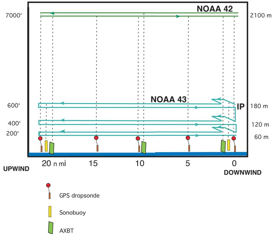
**Figure 7. CBLAST short stepped descent pattern (racetracks) in upwind / downwind and cross wind directions.**
