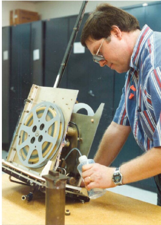
FIG. 7. Bob Black tends to the FORMVAR instrument, which improved the quality of cloud physics data from the aircraft in the 1960s. [Source: Stan Goldenberg, NOAA.]
