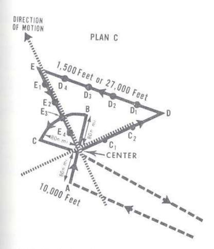
Used for tropical cyclones in the decay or rapid intensification stage to provide two 6-hour vortex fixes, with a special requirement for equivalent potential temperature data at 27,000 feet or sea surface temperature, sea level pressure, and wind data at 1,500 feet.
