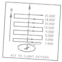
Preferred azimuth is through right front quadrant of the storm. Radial distance, r. from the eye is variable, i.e. 50 to 100 n.mi. Total pattern =
