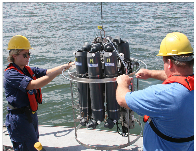
Figure 15. Top: R/V Hildebrand forward view. Middle: R/V Hildebrand aft view showing A-frame. Bottom: Seabird Rosette/CTD instrument being deployed from the R/V Hildebrand by NOAA scientists LT R. Kotkowski and C. Featherstone.
