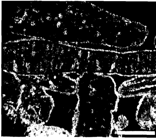
Figure 3: Cross polarized photomicrograph of beachrock from well H-2. Although appearing only slightly cemented, SEM analysis reveals these allochems to be well covered with a high Mg-calcite cement. Bar is 0.2 mm.
