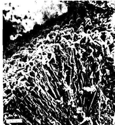
Figure 6: Scanning Electron Microscope photo of beachrock from H-5. Note the two generations of cements: 1) aragonite needles and 2) equant high Mg-calcite crystals. Bar is 10 micrometers.
