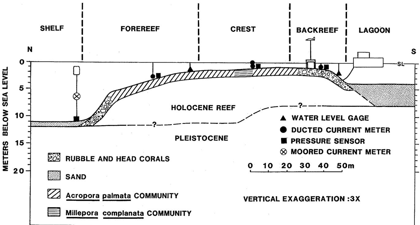
Figure 2. Typical instrument-deployment scheme used in the study of physical processes in reef systems at both Great Pond Bay and Tague Bay. This profile is from Tague Reef
