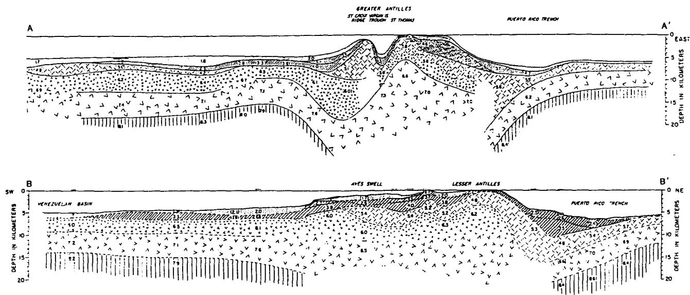
**Figure 4.** Refractor sections AA' and BB' located in Figure 3. Numbers are p-wave velocities in lon/sec., (from Officer *et al.*, 1959).
