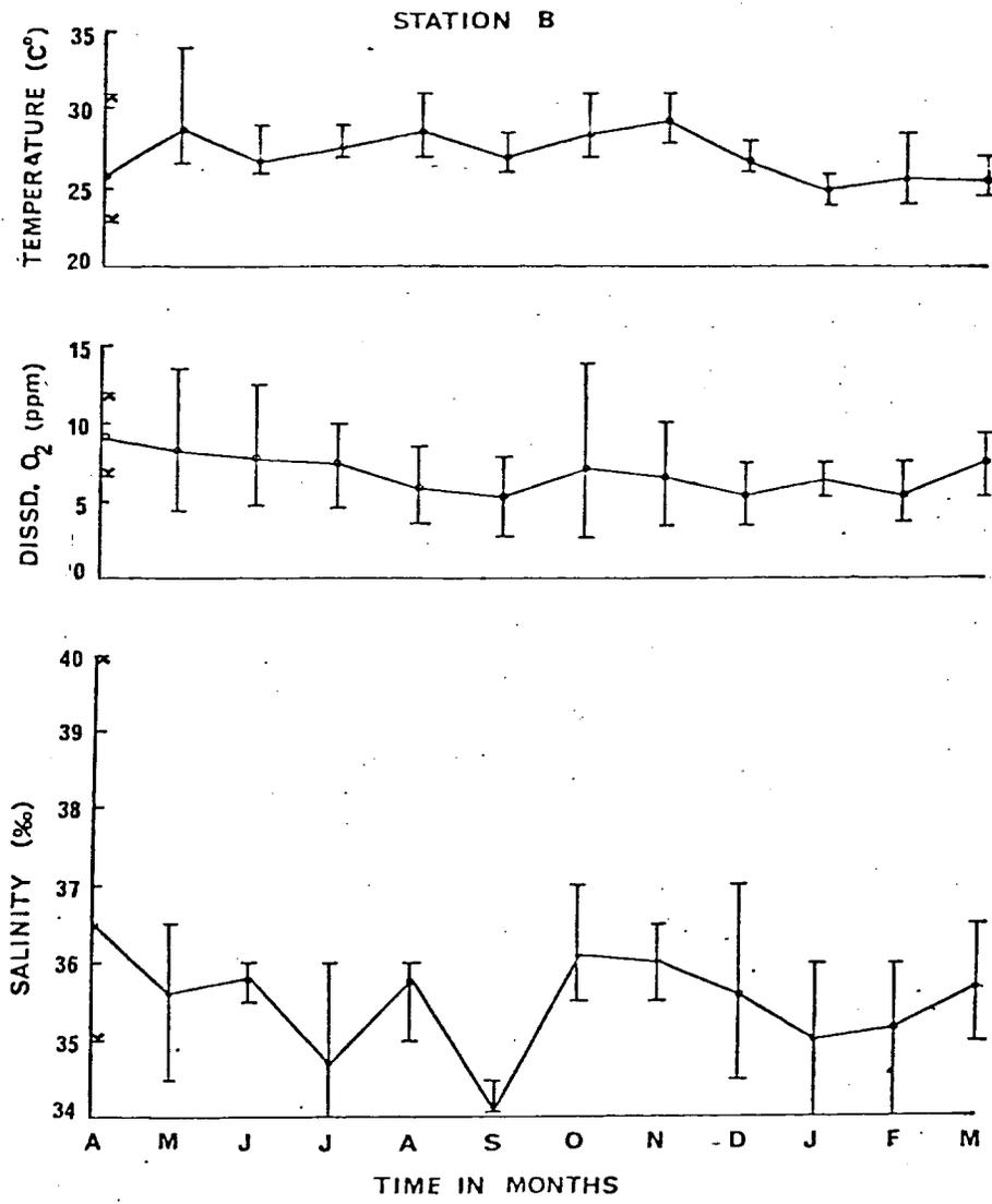
Fig. 17. Results of the twenty-four hour continuous monthly measurements of temperature, dissolved oxygen and salinity at Station B, Turrumote Reef between April, 1979, and March, 1980. • represents mean value, T and L, the highest and lowest values respectively
