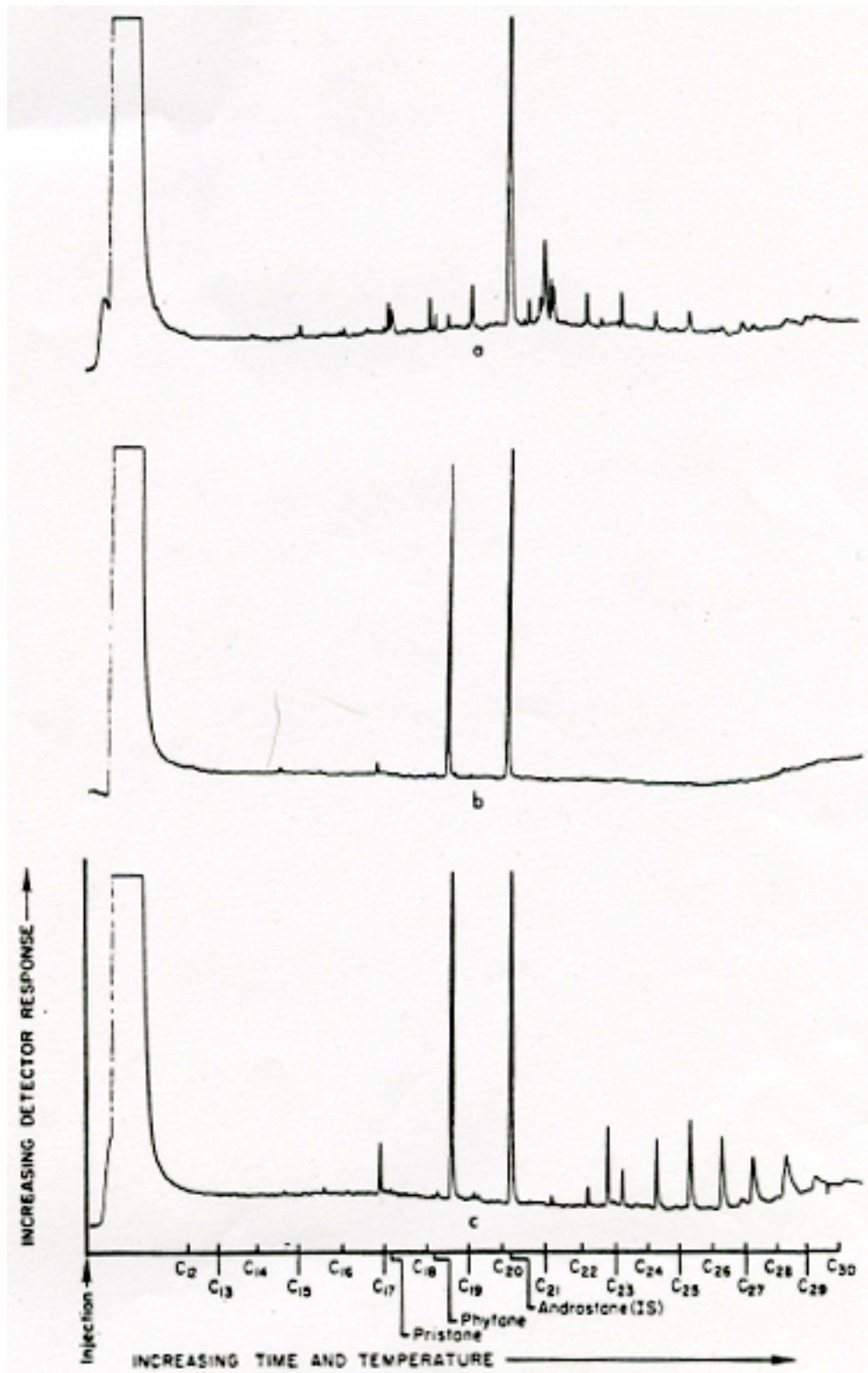
Figure 4. Chromatograms of aliphatic ( f_1 ) fraction. Interlaboratory calibration - offshore sediment samples - University of Miami.
