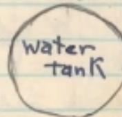
← 5'dia. a little wider at bottom. 5' high. On concrete blocks 3' off ground.
