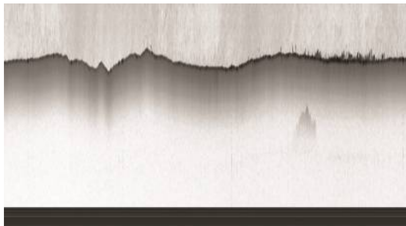
Figure 3.6. Sample of raw data file from the Bering Sea. The dark band near the top of the image is the water surface. Birds are seen just above the surface, and a school of fish is at the right. (Source: Churnside et al. , 2011b.)
