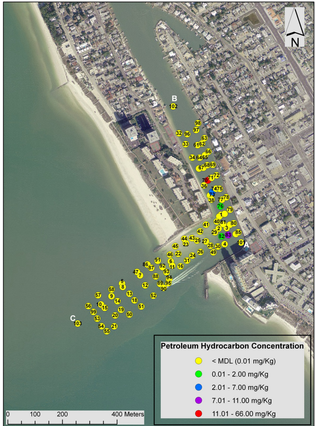
Figure 30: Spatial distribution of total petroleum hydrocarbons at the 0-99 cm depth interval in Blind Pass.
