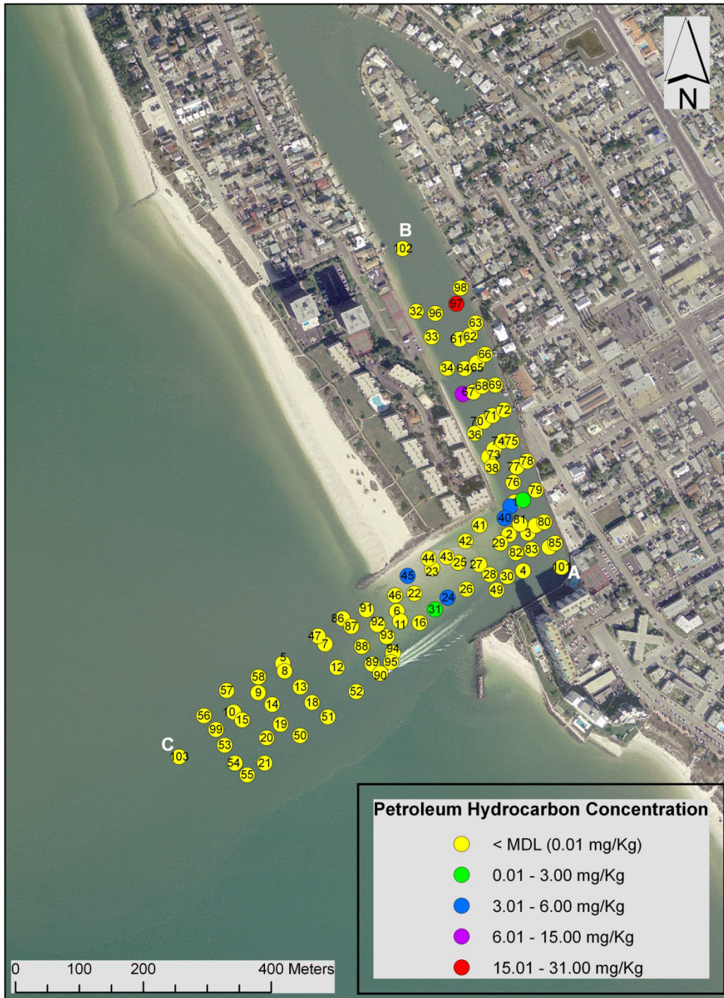
Figure 31: Spatial distribution of total petroleum hydrocarbons at the 100-199 cm depth interval in Blind Pass.
