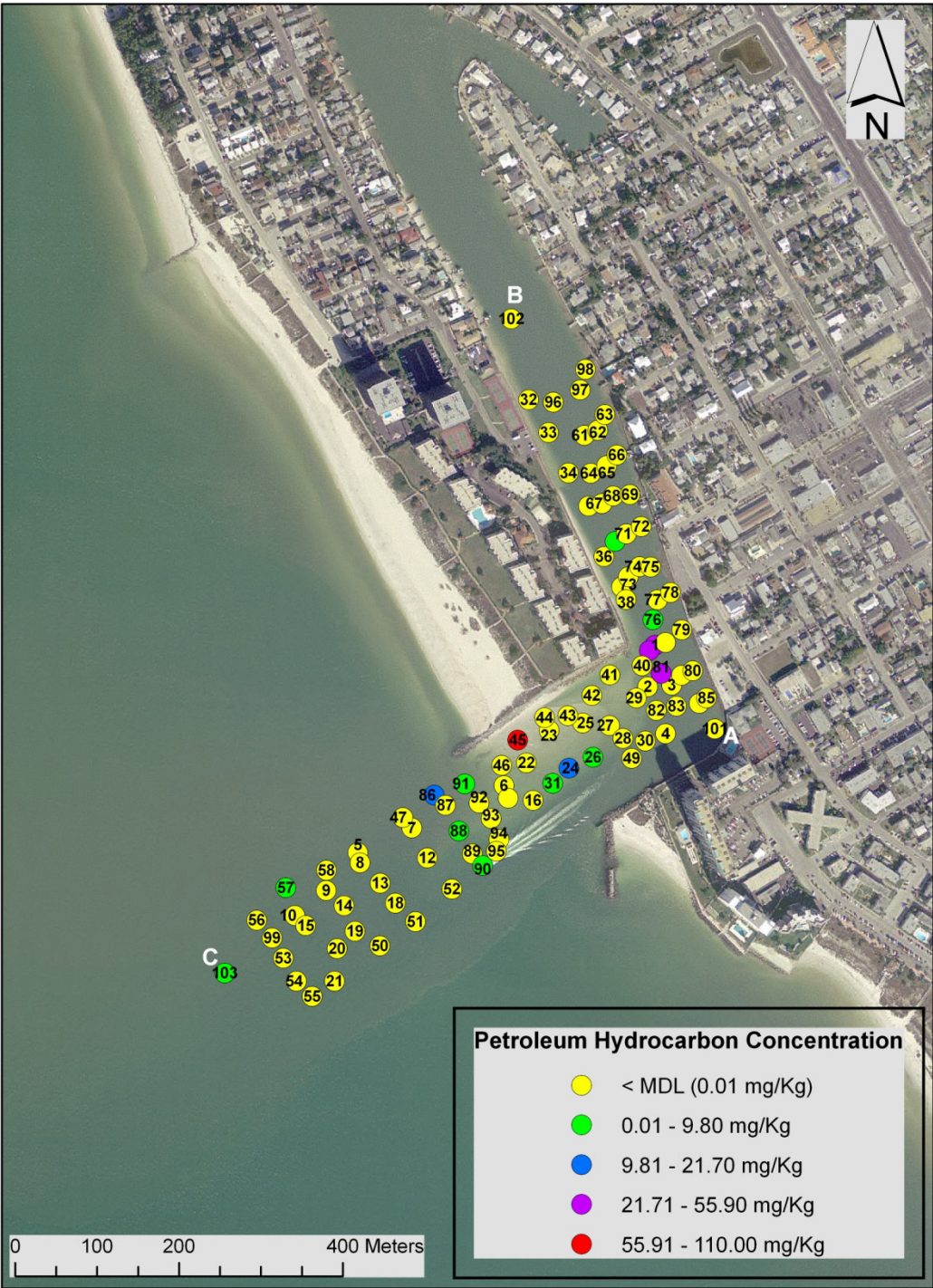
Figure 32: Spatial distribution of total petroleum hydrocarbons at the 200-299 cm depth interval in Blind Pass.
