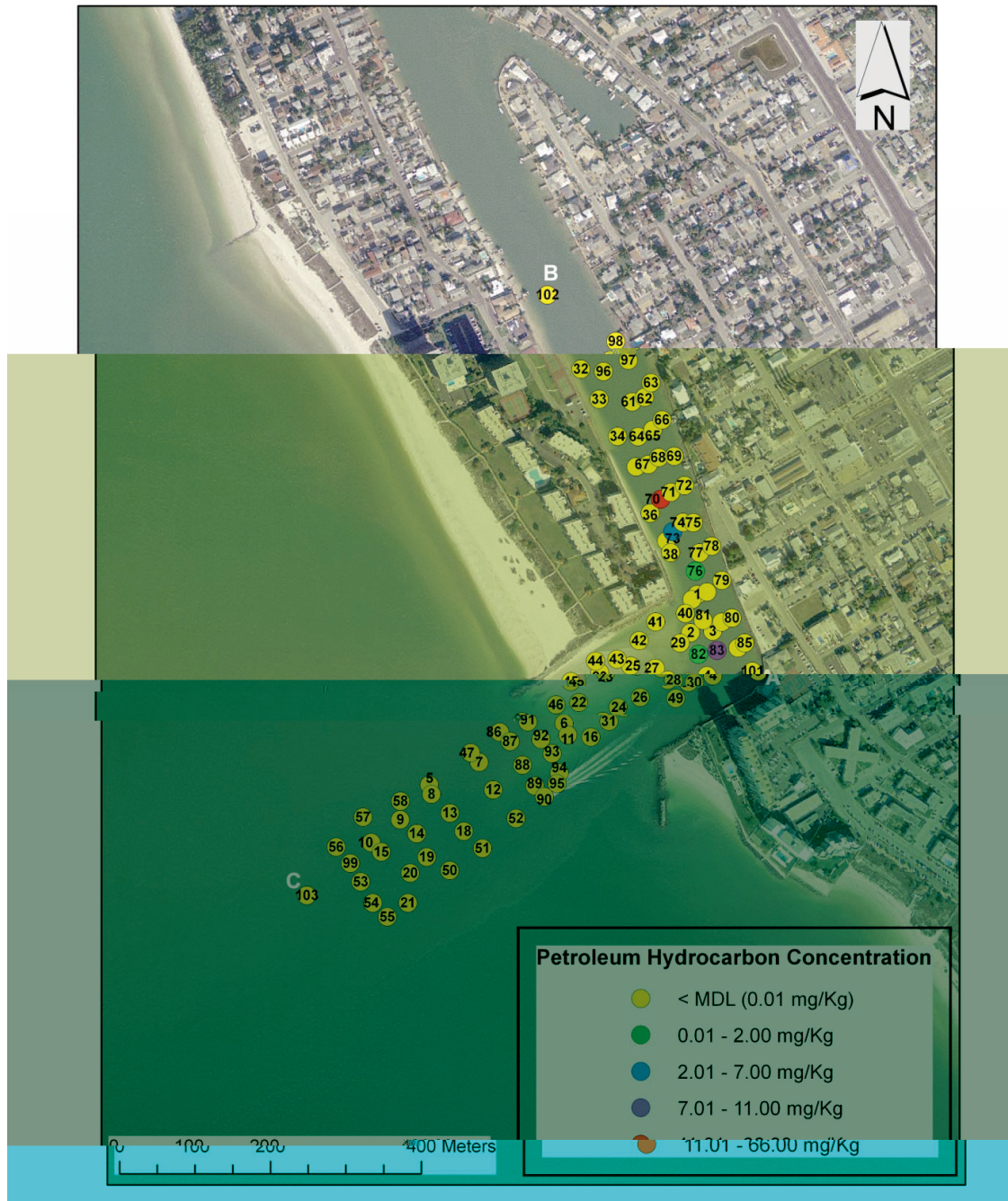
Figure 30: Spatial distribution of total petroleum hydrocarbons at the 0-99 cm depth interval in Blind Pass.
