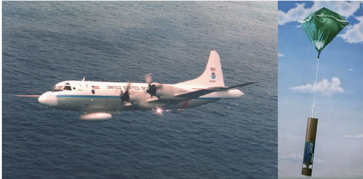
Fig. 6 L) One of two NOAA P3 hurricane research aircraft (Brad Smull). R) GPS dropsonde.
