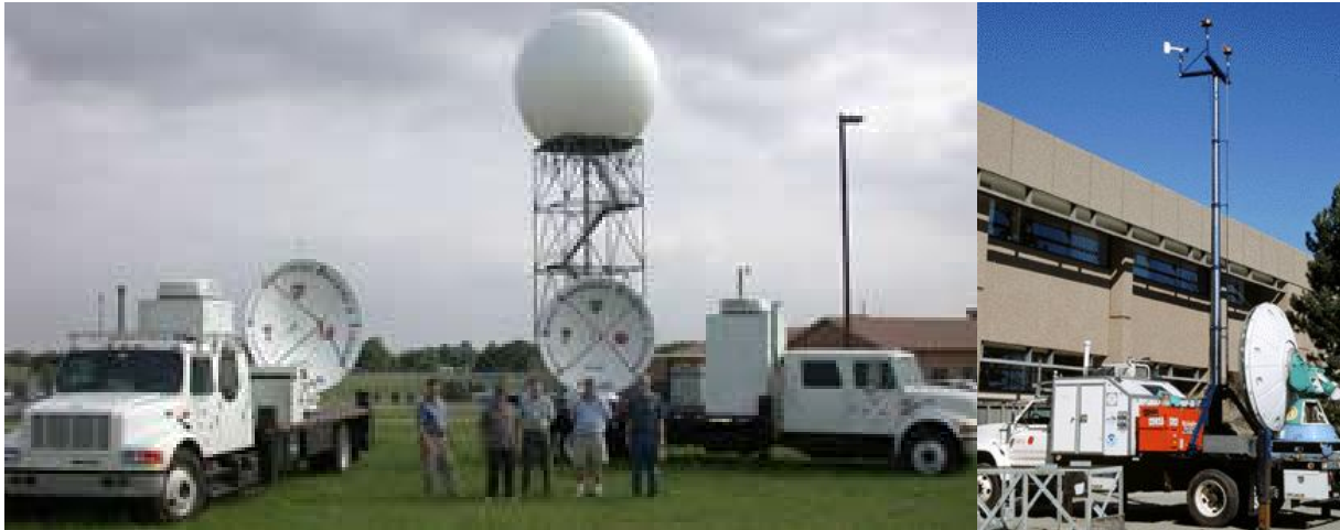
Fig. 3 L) Portable (SMART) Doppler radars with NEXRAD radar in background (NOAA/NSSL), R) Doppler on Wheels with telescoping anemometer mast (NCAR).
