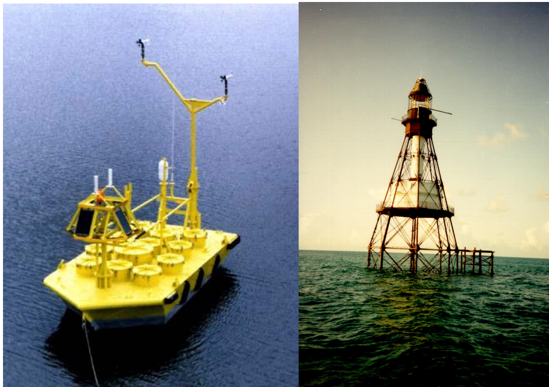
Fig. 4 L) NOAA moored buoy (6m Nomad ship hull, NOAA NDBC), R) Fowey Rocks C_MAN showing failed anemometer mast (extending horizontally to right, NDBC).
