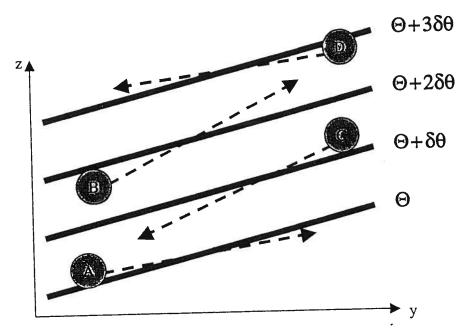
Baroclinic instability essentially is a slant-wise convection in a stably stratified fluid. The schematic above sketches four parcel trajectories (alphabetically labeled dashed arrows) relative to the zonal mean isentropic surfaces (heavy solid lines,  $\delta\theta > 0$ ). Note that all trajectories have a positive slope as the zonal mean isentropic surfaces. Please answer the following questions (estimated time: 60 minutes)
