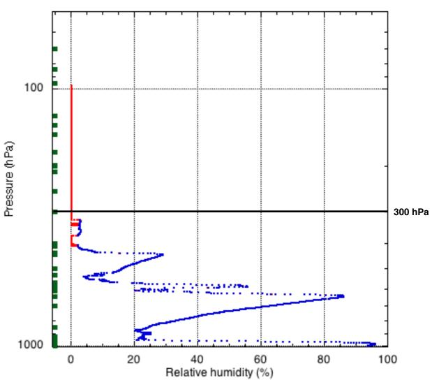
217 D-files from Global Hawk flight received 927,363 lines of data (4 Hz) 423,510 lines of humidity data (2 Hz) 67,581 lines have 0.1% relative humidity 1804 of these lines have 0.1% RH with no temperature 16% of the humidity data have synthetic information
