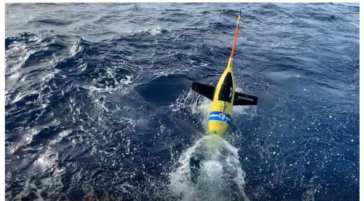
NOAA/AOML glider SG610 deployed in the tropical Atlantic during the 2020 Atlantic Hurricane Season
